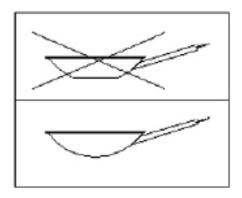
The generator does not accept unsuitable pots. Any other product not listed in this paragraph is automatically considered excluded and unsuitable for proper
