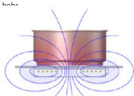
The basic principle of induction cooking is very simple. When the pot is placed on the ceramic surface of the hob, it enters the magnetic field generated by the induction system.
