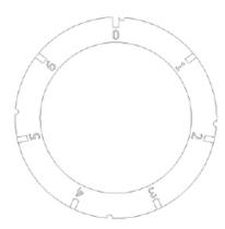
On the front panel, above the knob, a label marked with an index
